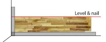
• For the installation of the second panel, follow the same process and procedures as outlined for the first panel. The only difference is the engagement/alignment of the decorative fillets. Simply line up the fillets and slide them together so that the wall panels blend-in giving the appearance of a continuous wall panel, or monolithic
